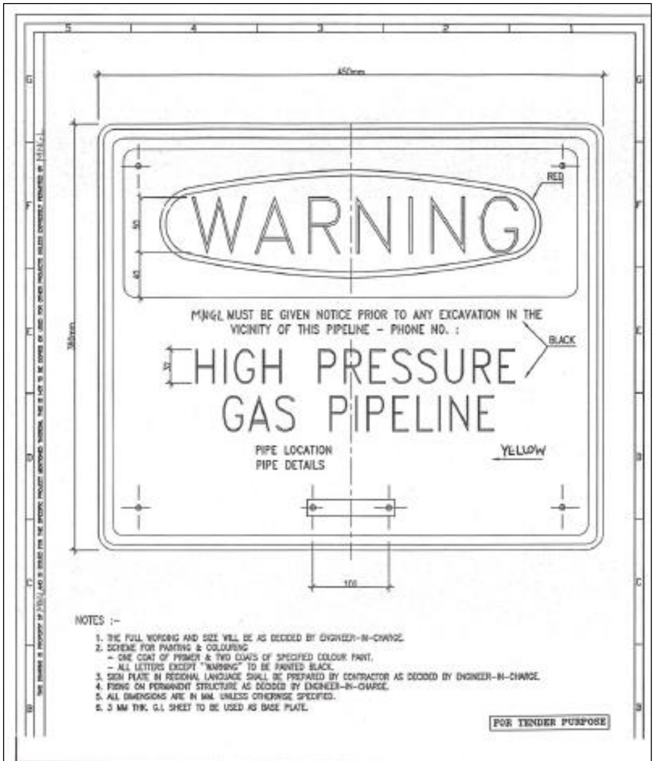
Warning Signs without foundation
