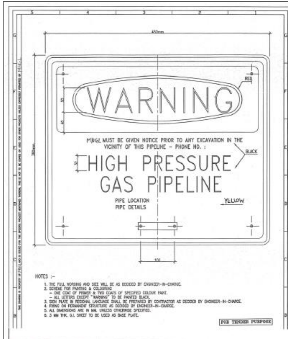
Warning Signs without foundation
